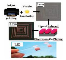
A photoassisted and inkjet-printed covalent polymer grafting method based on the photoreduction of aryldiazonium is presented. This powerful and versatile method to obtain local surface functionalization is combined with the ligand induced electroless plating process to obtain metal patterns onto flexible and transparent substrates with excellent mechanical and electrical properties, which may find applications in flexible electronics devices.
