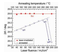
The effect of laser fluence on the crystalline nature of Ge<sub>2</sub>Sb<sub>2</sub>Te<sub>5</sub> films is studied in detail. Large structural differences between the laser-irradiated and thermally annealed films are revealed to be caused by the high heating rate and short duration of the laser pulse.
