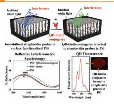
White light reflective interferometric spectroscopy and fluorescence measurements are used to implement a novel dual-mode optical porous silicon biosensor. Quantum dots act as signal amplifiers resulting in over an order of magnitude increase in sensor response and providing a secondary means of biomolecule-specific recognition through their distinct fluorescence spectra.
