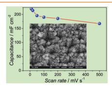
A hierarchical nickel compound (HNC) film is prepared using a facile, one-step, and binder-free method. The HNC demonstrates both large capacitance and superior rate capability. The capacitance reduction is only 24%, even when the scan rate is increased by 50 times. The HNC also exhibits an excellent cycle life.
