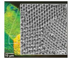
The cuticular photonic polycrystals formed by the beetle Entimus imperialis are a perfect example of a natural diamond-type triply periodic bicontinuous cubic structure with structural parameters that are optimized to open up the largest possible photonic stop gaps. Depending on whether the cuticular network is complemented by air or SiO<sub>2</sub>, the optical properties of individual domains vary from bright coloration to no coloration and transparency.
